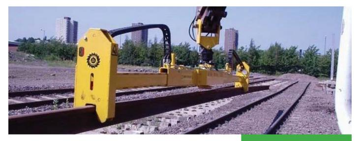
ur TRLB20 Telescopic Rail Beam is the first choice for handling new rails up to 65ft in length.
