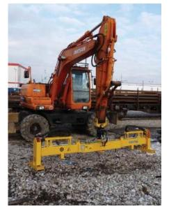
Max. Hyd Pressure 210Bar Min. Hyd Pressure 90 Bar Body Colour 08E51 Yellow Moving Parts Signal Red
